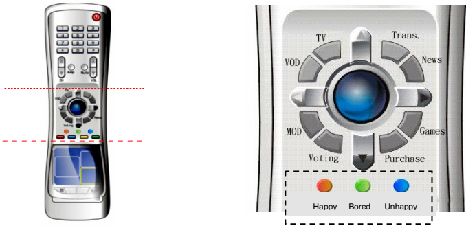
Fig. 1. Concept of remote control and mood input button
